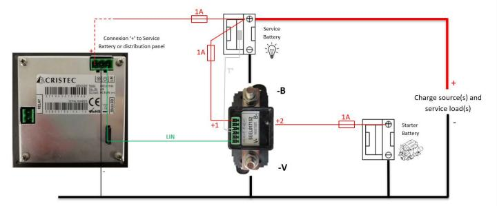
Monitoring of a service battery + voltage of the starter battery and control of the flow of a solar panel
